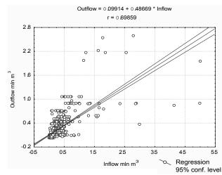
Fig. 5. Graphical presentation of the correlation between the volume of outflowing and inflowing water in the Słup Reservoir (Out res and In res), 2005-08.
