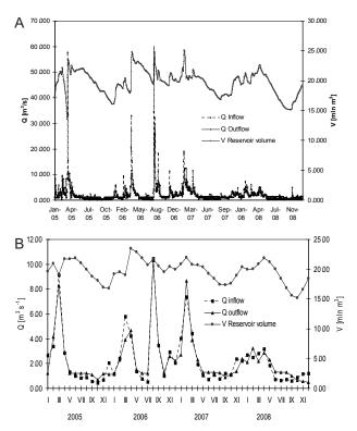
Fig. 3. Daily (A) and monthly (B) inflow and outflow values and the volume of the Shup Reservoir in 2005-08.
