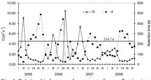
Fig. 4. Relationship between the amount of water flowing into the Shup Reservoir and reservoir capacity in a given time vs. changeability of the retention time, 2005-08.
